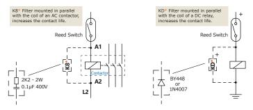
**? Risk of failure (welding of the Reed Switch Contact)** due to CAPACITANCE, which can occur depending on the distance and cable used in the connection to the contactor.
