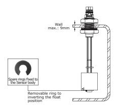
Removable ring to inverting the float position
